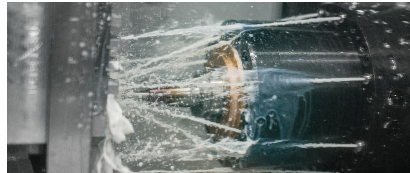
The 24,000-rpm spindle and improved part accessibility of the a61nx-5E have improved cycle times by 80 percent over previous technologies.
