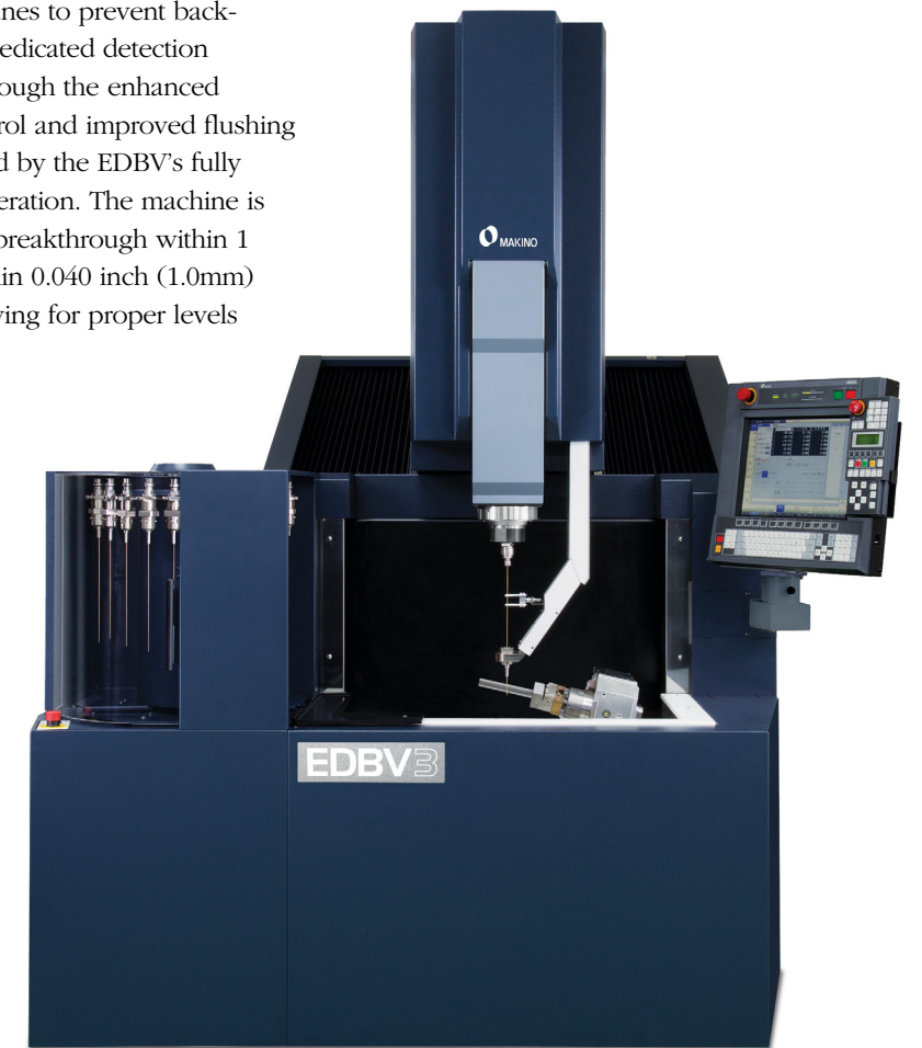
All EDM drilling on EDBV machines is performed fully submerged under water. This approach enables faster machining speeds, improves part quality, and creates more stable and consistent conditions during cavity wall penetration.
