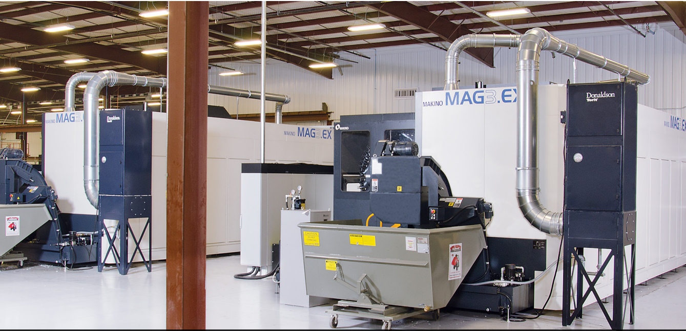
In late 2014, Dynamic purchased two MAG3.EX 5-axis HMCs to begin producing complex monolithic aluminum structural parts.
